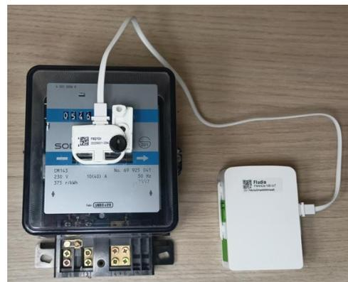
The optical head starts measuring and instructs the FM442e radio/battery box to connect to the network.
