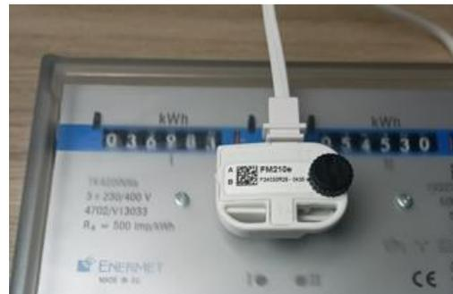
If it is an **electromechanical meter**, make sure the optical head is properly attached to the adhesive plastic mount with the help of the black screw:
