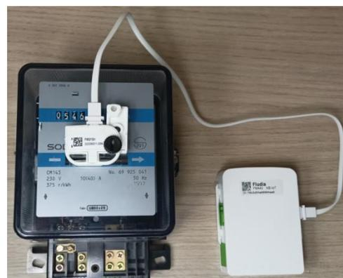
The optical head starts measuring and instructs the FM442ir radio/battery box to connect to the network.
