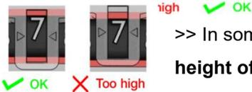
>> In some cases, the digit can be higher or lower than normal. Position the arrows at **mid-height of the frame, not at mid-height of the digit**.
