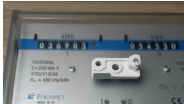
Then, position the optical head on top of the plastic mount and tight the black screw.
