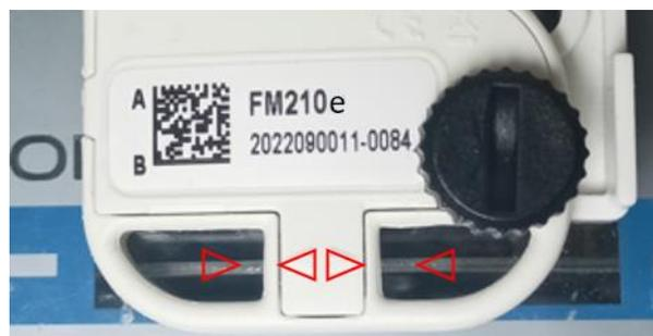
If the arrows are not completely lined up with the disc, loosen the screw, adjust position, and tighten the screw.
