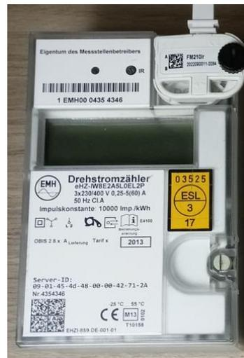
If it is an **electromechanical meter**, make sure the optical head is properly attached to the adhesive plastic mount with the help of the black screw:
