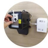
**BelSenso FM332Log** is a datalogger recording electricity consumption at the main electricity meter level. It can be installed in all types of buildings.
