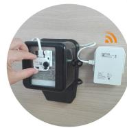
**BelSenso FM432e** is a universal device that provides Automatic Reading features to all types of electricity meters. The interoperability with the IoT LoRaWan networks, dedicated to Connected Objects, allows to be quickly informed of the level of electricity consumption. The ideal device to deploy energy efficiency services for Small and Medium Buildings.
