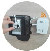
**BelSenso FM432ir** is a universal IoT optical sensor that can read many types of Electricity Meters. It has been designed for Meters with infrared communication ports, but can also be used with old Ferraris meters. Radio transmission is based on LoRa technology (Long Range and low consumption) and is compatible with existing LoRaWAN networks.
