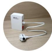
The FM442e is a plug-and-play IoT sensor designed for monitoring electricity consumption in all types of buildings. The optical head can be quickly attached to the main electricity meter or a submeter, and the NB-IoT/LTE-M modem connects through standard cellular networks. Measurement data is transmitted to an MQTT broker and can be retrieved by any EMS (Energy Management System).
