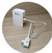
The **FM442g-n** is a plug-and-play IoT sensor designed for monitoring gas consumption in all types of buildings. The optical head can be quickly attached to the main gas meter, and the NB-IoT/LTE-M modem connects through standard cellular networks. Measurement data is transmitted to an MQTT broker and can be retrieved by any EMS (Energy Management System).
