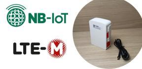
The **FM442p-n** is a plug-and-play IoT sensor designed for monitoring energy consumption in all types of buildings. It can be connected to all kinds of meters featuring a pulse output (water, gas, heat, electricity). The NB-IoT/LTE-M modem connects through standard cellular networks. Measurement data is transmitted to an MQTT broker and can be retrieved by any EMS (Energy Management System).
